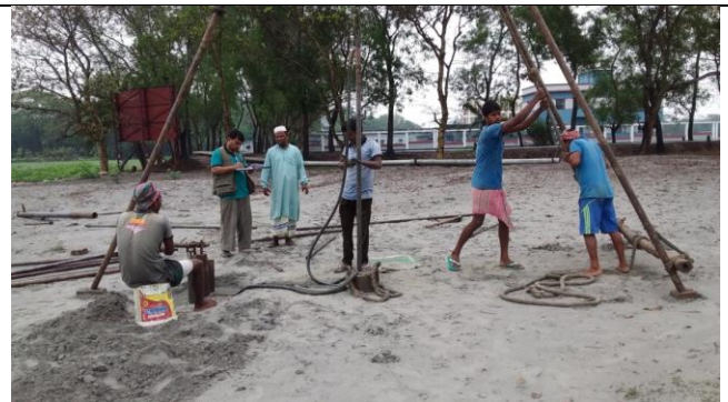
Plate-2.2: Subsurface sediment collection by SPT method at Baher Char, Rangabali, Patuakhali.
